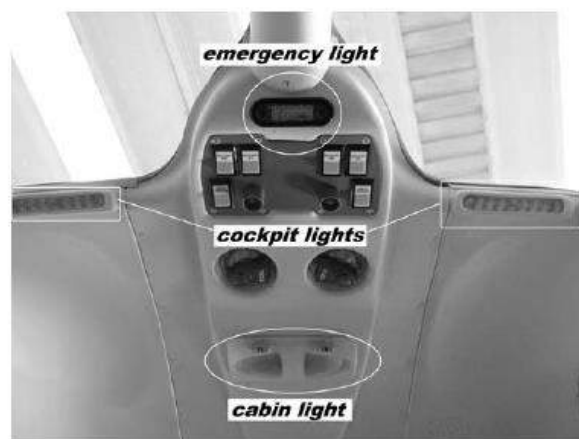
Figure 9. – Over-head panel lights arrangement
