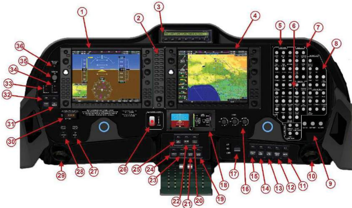
GARMIN G1000 NXi - Instruments panel (typical layout)
