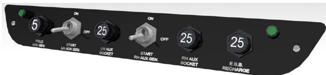
LH breakers rack: built-in generators field switches and system related breakers (panel type 2)
